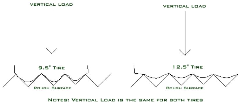
**Mechanical Keying:** This is the second critical benefit of a narrower tire. As the vertical load increases, so does the compression and flexing of the tires tread and rubber to the surface protrusion. A narrower tire generates greater vertical load on the rubber and the tread, increasing tread compression in conformance to the surface irregularity. A wider tire in contact with more surface conforms less, and will shear sooner than a narrow tire.
